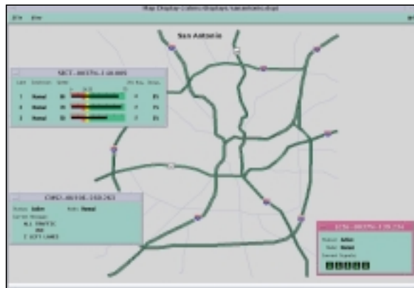
Supported by SwRI internal funding, software engineers converted standard GIS data files into a format more easily displayed and manipulated on ATMS displays.
