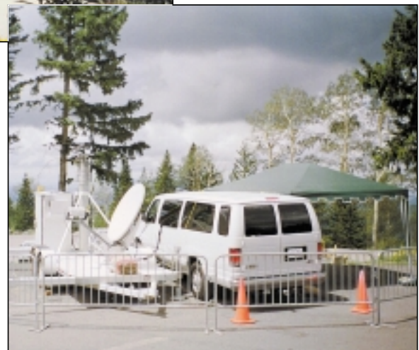
Institute engineers designed a remote incident-management system that uses satellite communications to provide command and control capability for rural ITS applications.
